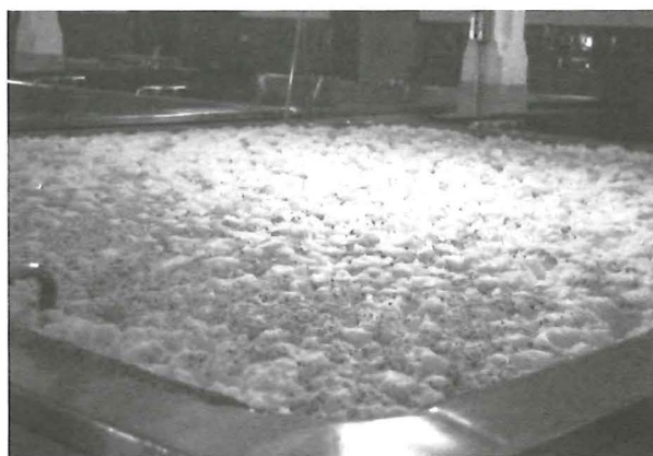
Large open fermenters at the Feldschlösschen Brewery, Switzerland. Feldschlösschen actually brews using very large unitanks holding thousands of barrels of beer, but they also use the older open fermenters for test batches.
