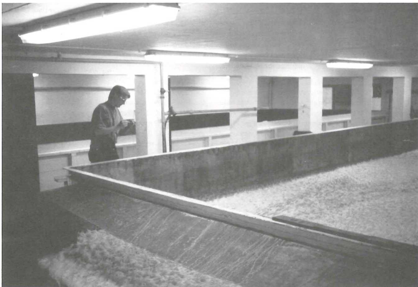
Jim Busch is harvesting a yeast sample from an enormous copper open fermenter at Liefmans Brewery in Oudenaarde, Belgium. This shot was taken two days after the yeast was pitched. The day after the trub is run off, the brewer harvests the clean yeast for subsequent pitchings. Note the open fermenter where the trub is being run off: Wooden boards are placed over the end when the fermenter is not being skimmed.
